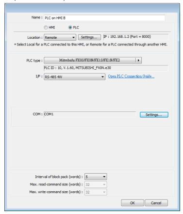
Create a Set Bit Object, select "PLC on HMI B" in [PLC name] to control the PLC connected with the remote HMI B.
